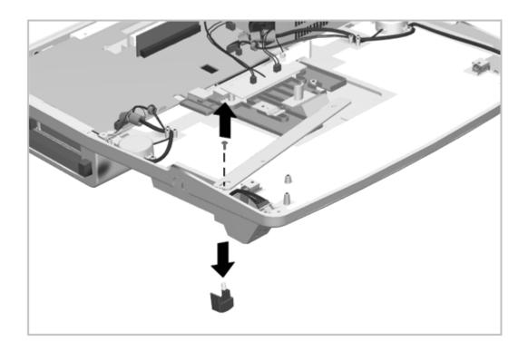
Figure 6-35. Removing the Docking Lever
